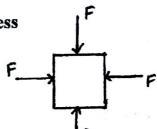
When a deforming force acts normally and uniformly all over the surface of a body, then the restoring force for unit area of the body is called volume stress or bulk stress.
