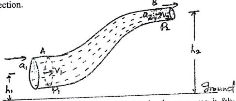
A&B are two sections of the pipe. Let P1 &P2 be the pressures, h1&h2 be mean heights , a1&a2 the areas of cross section and v1 &v2 be the velocities of flow at the sections A&B respectively.
