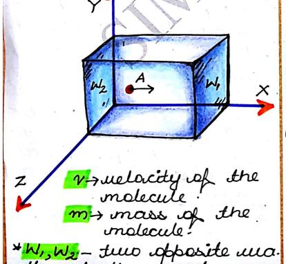
A-> molecule mouing alo ing x - idivection. inside la rubical meusel up writ uside. A molecule (A), moung along x-direction hits the wall W, and rebounds with same welecity. momentum of the molecule before collision = my retic theory temperature momentum of the molecular of the indecution is in its in meal of the indecution in the indecution of the indecution of the indecute of the igas.
