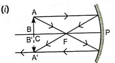
Nature of image: Real, inverted and same size image is formed at the centre of curvature.
