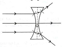
Thus, because of the concave shape of both the faces, the double concave lens diverge the rays of parallel beam of incident light.
