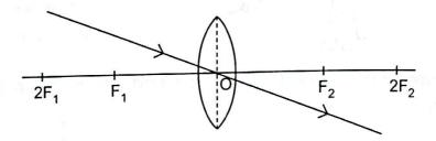
8. Redraw the given diagram and show the path of the refracted ray:
