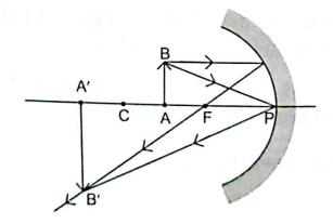
10. Which kind of mirrors are used in the headlights of a motor-car and why? [Foreign] Ans. Concave mirror, to get the parallel beam of light.
