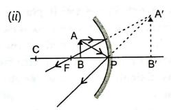
Nature of image: Virtual, enlarged and erect image is formed behind the mirror.
