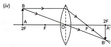
Nature of image: Real, inverted and size to size, image is formed at 2F on the other side of lens.
