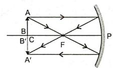
Since, |v| = |u| = 2f, it means that the object is placed at the centre of curvature (C) of a concave mirror, the image formed is at the centre of curvature, real and inverted and of the same size as the object.
