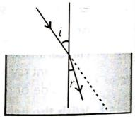
i =Angle of incidence r =Angle of refraction
