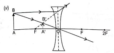
Nature of image: Virtual, erect and diminished image is formed between O and F on the same side of object.
