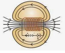
In the above figure, when the north pole of a bar magnet is brought near the end connected to the negative terminal of the battery, the solenoid repels the bar magnet. Since like poles repel each other, the end connected to the negative terminal of the battery behaves as the north pole of the solenoid and the other end behaves as a south pole. Hence, one end of the solenoid behaves as a north pole and the other end behaves as a south pole.
