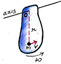
vigid bedy votating about an axis passing through 0 with uniform angular vielocity w. The body consists of in ru mber of particles. Let une particle of mass m is set nated 'at a idis tance 's from cases of votation: Linear mélocity of the particle V=rw violation: kinectic energy of particle = 1my2  $= l_{2}m\pi^{2}\omega^{2}$ K.E. of whole body =  $E \pm m H^2 w^2$
